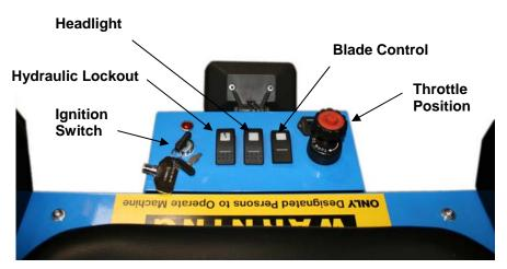
Figure 2 Operator Controls - Drivers Seat
